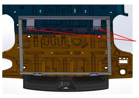
(1) Assemble mounts to frame as shown. Place mounts over standard factory threaded holes (only outside holes on mounts are utilized they may have black tape over them), and install 3/8-16 x 1" bolts
