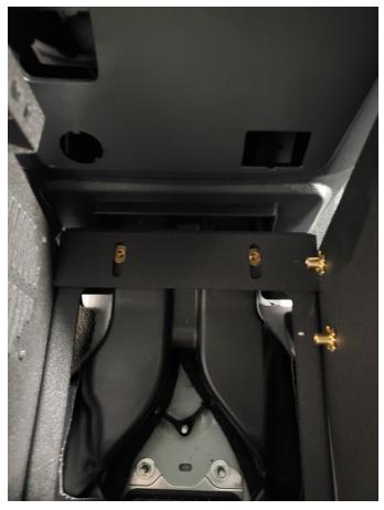
Install factory rear air if applicable into supplied faceplate with supplied spacers and hardware
