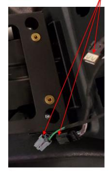
Install console over new floorplate, and slide forward towards dash until it seals up against it. Install two 1/4-20 BHCS in the front slot location and two 1/4-20 BHCS in the rear armrest area securing the console to the floorplate.
