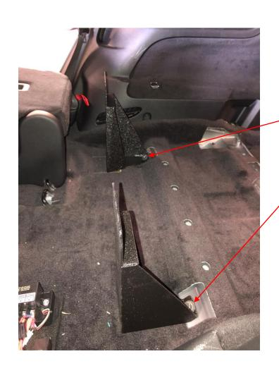
UTILIZE FACTORY MOUNTING LOCATIONS TO INSTALL FEET INTO VEHICLE.
