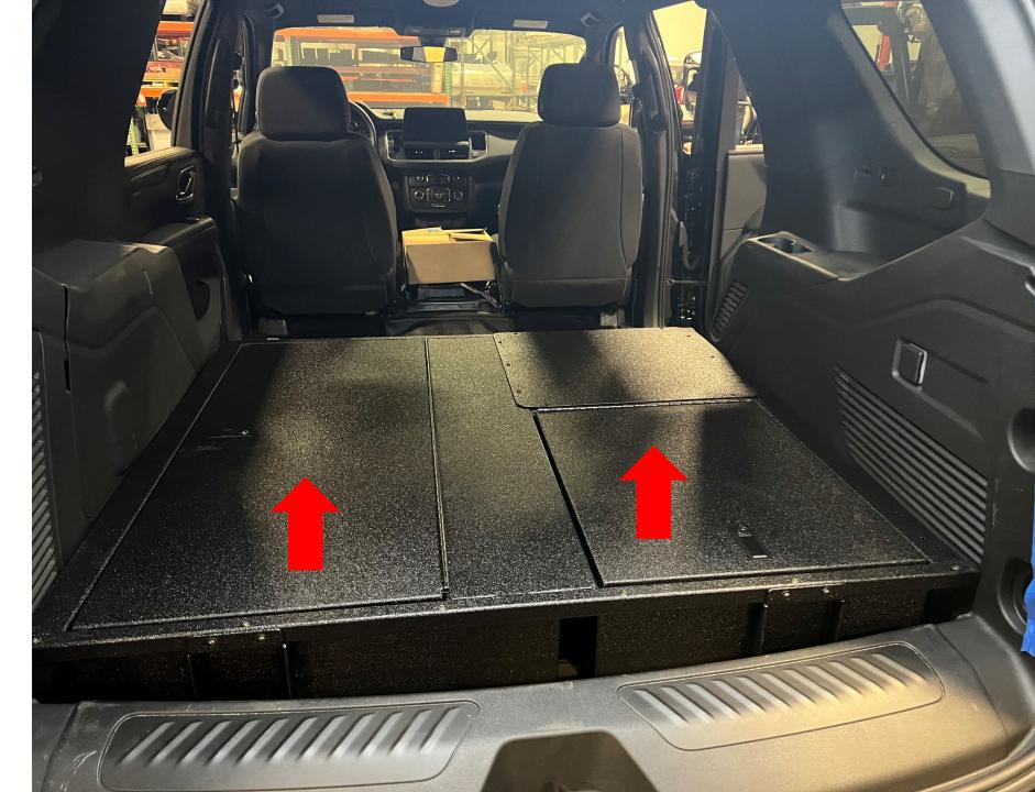
INSTALL PROVIDED 10/32 SCREWS INTO SLOT LOCATIONS ON MOUNT INTO FLOOR. THERE WILL BE A TOTAL OF 4 SCREWS, 2 PER SIDE. TIGHTEN SCREWS TO FLOOR.
