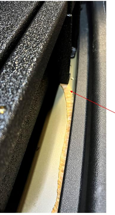
PENCIL A MARK WHERE THE HOLES ON THE MOUNTS MEET THE FLOOR OF THE VEHICLE. YOU WILL BE DRILLING OUT FOR A NUTSERT USING A 7/16" DRILL BIT.
