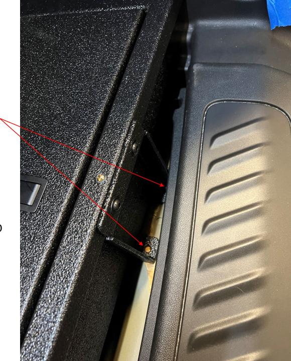
SLIDE FLOOR TOWARD FRONT ON MOUNTS, REMOVE THE RUBBER FROM THE VEHICLE FLOOR, AND DRILL AND INSTALL NUTSERTS INTO VEHICLE FLOOR. REMOVAL OF REAR LOWER TRIM WILL MAKE THIS EASIER.
