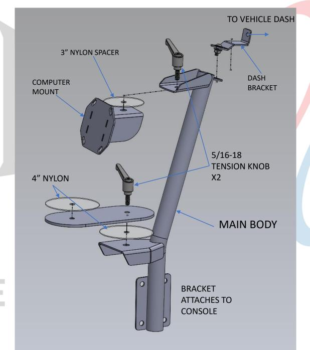
1X MAIN BODY 1X DASH BRACKET 1X TABLET MOUNT 1X PIVOT ARM 2X 5/16-18 TENSION KNOBS 5X ¼-20 BHCS 6X 1/4" WASHERS 1X ¼-20 KEP NUTS 2X 4" NYLON SPACERS 1X 3" NYLON SPACER
