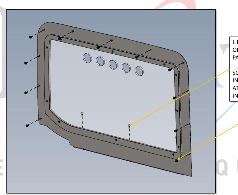
LINE UP BOTTOM FLANGE ON TOP OF DOOR OPENING, AND ALIGN PANEL IN WINDOW FRAME.
