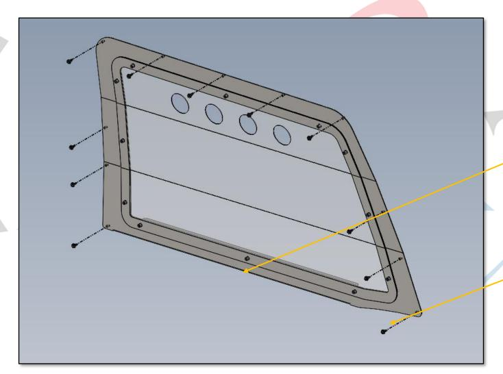
LINE UP BOTTOM FLANGE ON TOP OF DOOR OPENING, AND ALIGN PANEL IN WINDOW FRAME.
