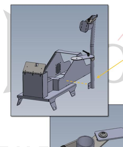
ATTACH TO CENTER CONSOLE USING 2X ¼-20 BHCS W/WASHERS.
