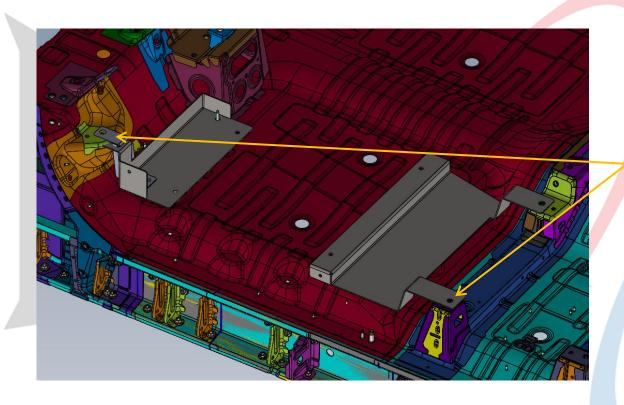
PLACE LOWER SHELF SKIN ON MOUNTING BRACKETS, ALIGN WITH HOLES ON BRACKETS, PLACE LIP FLUSH WITH OUTSIDE OF BRACKET REMOVE REAR SEAT, LIFT FRONT SEAT FROM REAR MOUNTING POINTS.
