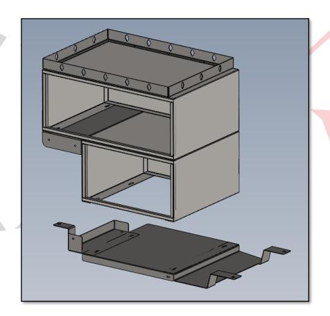
MOUNT CUBBIES ON BRACKETS AND SECURE WITH PROVIDED HARDWARE, ADJUST BOTTOM SKIN INTO POSITION AND TIGHTEN MOUNTING HARDWARE.
