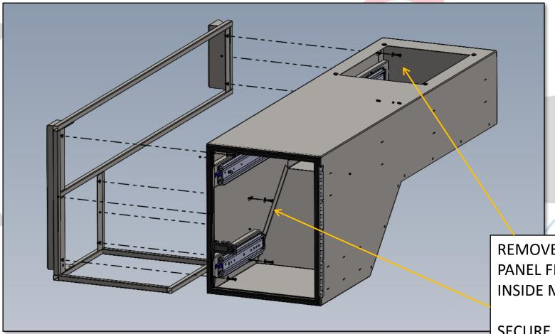
REMOVE DRAWERS AND UPPER ACCESS PANEL FROM BOX TO ACCESS INSIDE MOUNTING HOLES
