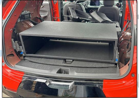
INSTALL DRAWER INTO BOX TO COMPLETE INSTALLATION.
