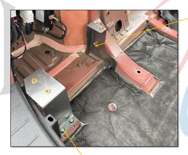
INSTALL REAR BRACKETS WITH 10MM BOLTS & WASHERS PROVIDED
