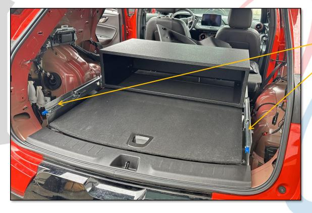
EXTEND SLIDES TO FULL OPEN AND ATTACH SMALL RAILS AS SHOWN USING 10-32 BHCS PROVIDED. SLIDE BOX FORWARD TO CHECK OPERATION, ADJUST SLIDE BRACKETS AS NEEDED.
