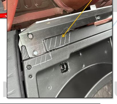
REMOVE SCREWS FROM HINGES ON SPARE TIRE COVER PANEL
