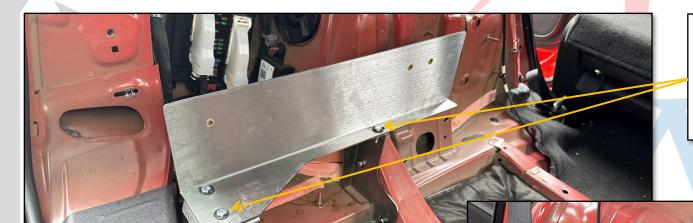
INSTALL SLIDE RAIL BRACKETS ON FEET AS SHOWN, USING SUPPLIED ¼-20 BHCS NOTE ORIENTATION OF BRACKETS FOR CORRECT INSTALLATION
