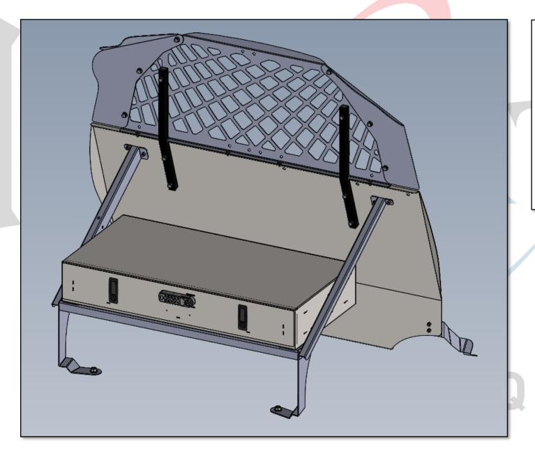
INSTALLATION OF HKG MOUNTING FOOT AND BOX WITH JOTTO CAGE IN DURANGO
