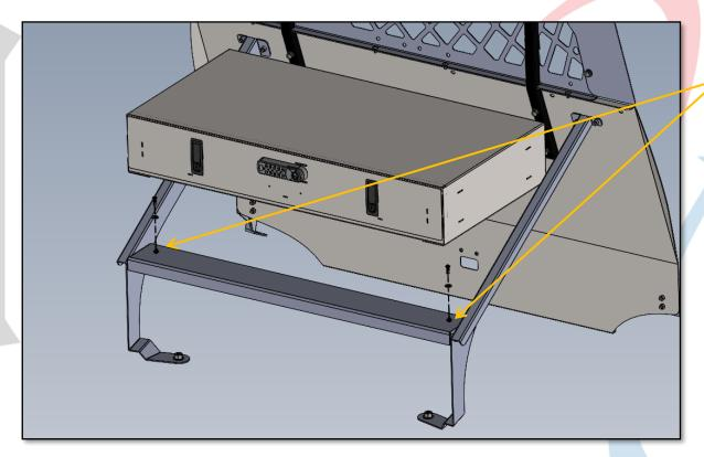
TO MOUNT BOX ON BRACKET, DRILL HOLES AS NEEDED FOR MOUNTING POINTS, INSTALL PROVIDED 1/4-20 NUTSERTS INTO BRACKET
