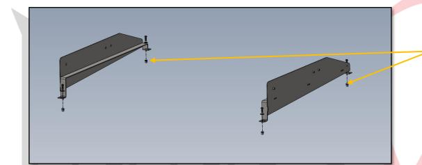
MOUNT BRACKETS TO VEHICLE USING PROVIDED HARDWARE, DO NOT COMPLETELY TIGHTEN SCREWS AT THIS POINT
