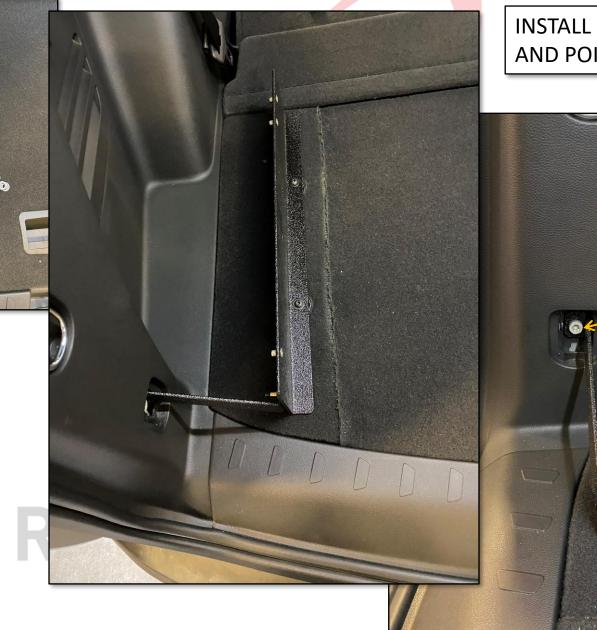
INSTALL BRACES AS SHOWN TO BRACKETS AND POINTS SHOWN ON VEHICLE
