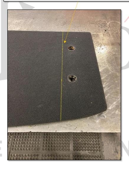
RE-INSTALL LID, REMOVE LID HINGES, AND CUT OUT CENTER FOR SPARE TIRE ACCESS LID WILL SIT ON FRONT AND BACK LEDGES
