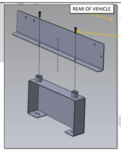
USE 1-1/2" ¼ -20 BOLTS & WASHERS TO SECURE SLIDE RAIL BRACKETS
