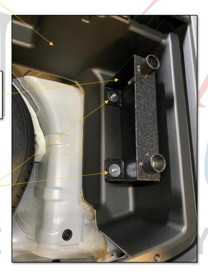
INSTALL LID AS SHOWN AND MARK FOR CUTTING, LOWER LID AND TAP LIGHTLY WITH HAMMER TO INDENT TAPE TO MARK FOR CUTTING HOLES.
