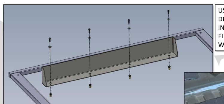
USING MOUNTING FOOT AS A GUIDE, DRILL AND INSTALL (4) ¼-20 NUTSERTS IN VEHICLE FLOOR. BOLT MOUNT TO FLOOR USING ¼-20 BOLTS AND WASHERS.
