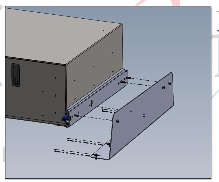
INSTALL LOCKING SLIDES TO BRACKETS, AND MOUNT BOX TO SLIDES
