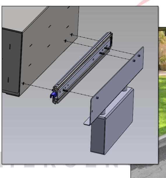
INSTALL LOCKING SLIDES TO BRACKETS, AND MOUNT BOX TO SLIDES
