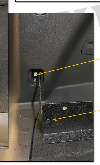
EXISTING VEHICLE HARDWARE IS RE-USED TO ATTACH BRACKETS AS SHOWN
