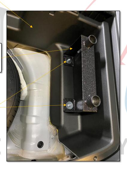
INSTALL LID AS SHOWN AND MARK FOR CUTTING, LOWER LID AND TAP LIGHTLY WITH HAMMER TO INDENT TAPE TO MARK FOR CUTTING HOLES. CUT WITH 1-1/2" HOLE SAW.
