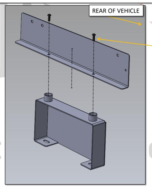
INSTALL BRACES AS SHOWN TO BRACKETS AND POINTS SHOWN ON VEHICLE
