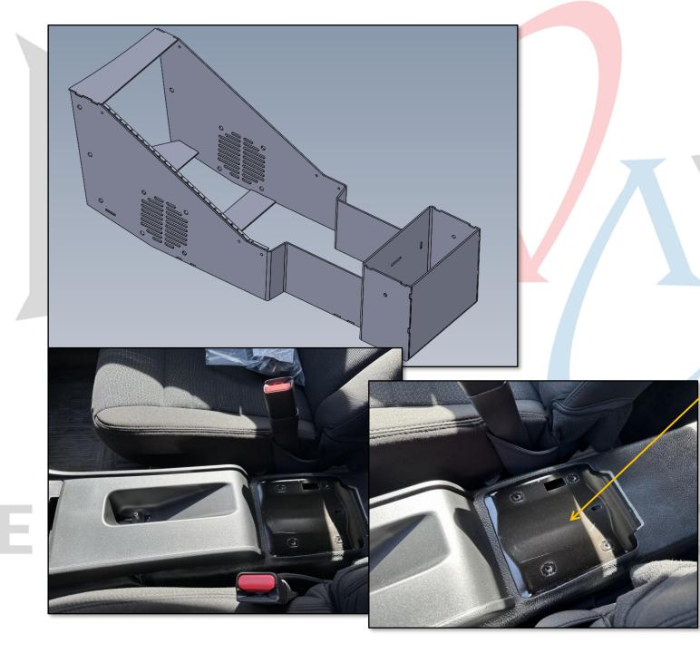
INSTALLATION OF CONSOLE WITH MOUNTING PLATE
