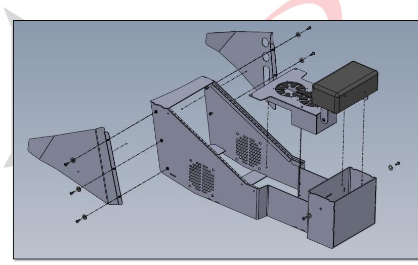
USING PROVIDED HARDWARE, ATTACH SIDE WINGS, CUPHOLDER, AND ARMREST
