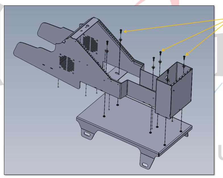
USING PROVIDED HARDWARE, ATTACH CONSOLE BODY TO FLOOR PLATE
