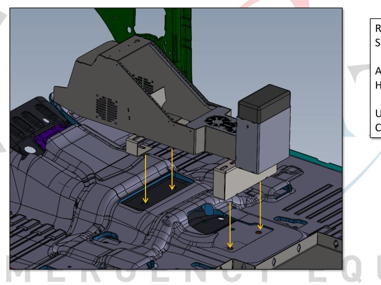
REMOVE FACTORY CONSOLE IF NEEDED, SET ASIDE FACTORY HARDWARE
