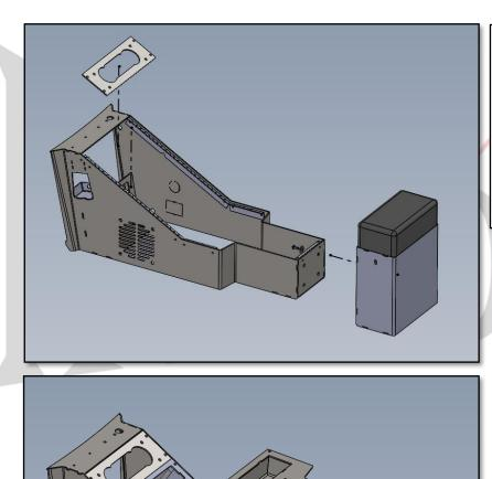
INSTALL A/C FACEPLATE AND MOUNT ARMREST USING PROVIDED HARDWARE. INSTALL CUPHOLDER/TRAY UNIT AND SECURE TO RAILS WITH PROVIDED HARDWARE.
