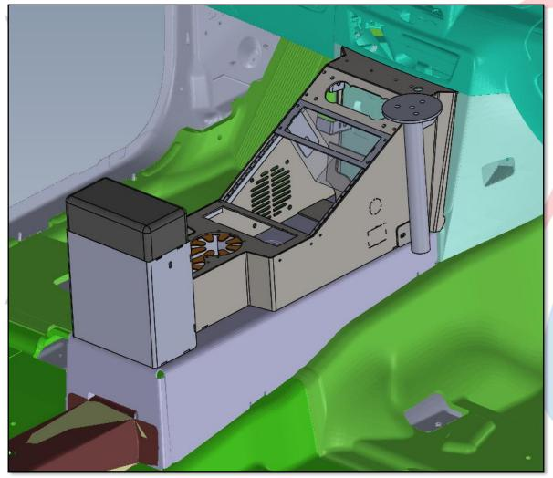
INSTALLATION OF DUAL NOTCH CONSOLE WITH FACTORY FLOOR PLATE
