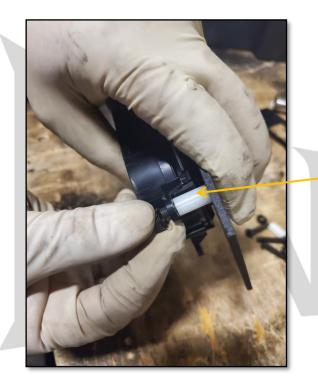
INSTALL A/C CONTROLS IN PROVIDED FACEPLATE USING PROVIDED SPACERS AND HARDWARE.
