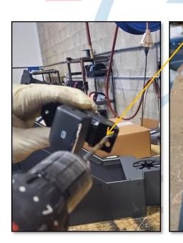
INSTALL PARKING BRAKE SWITCH: DRILL OUT MOUNTING HOLES SHOWN TO 3/16" ATTACH SWITCH TO BRACKET SHOWN WITH INCLUDED HARDWARE.
