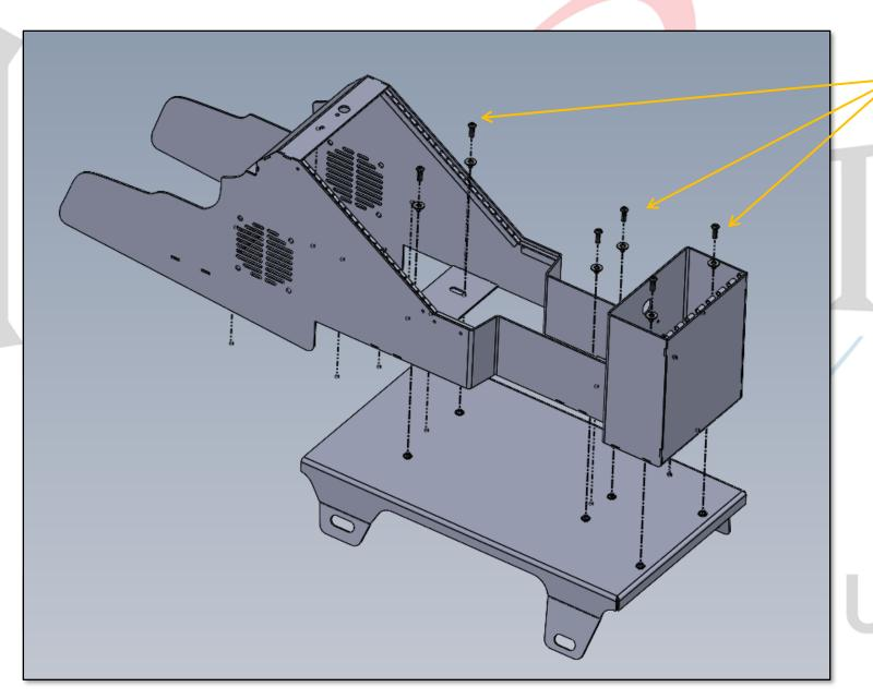
USING PROVIDED HARDWARE, ATTACH CONSOLE BODY TO FLOOR PLATE
