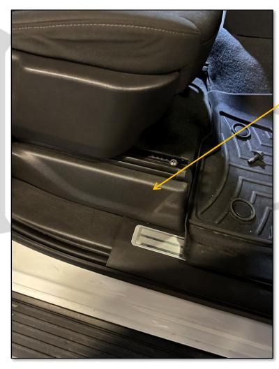
REMOVE SIDE TRIM PANELS ON FRONT SEATS, BOTH DRIVER AND PASSENGER
