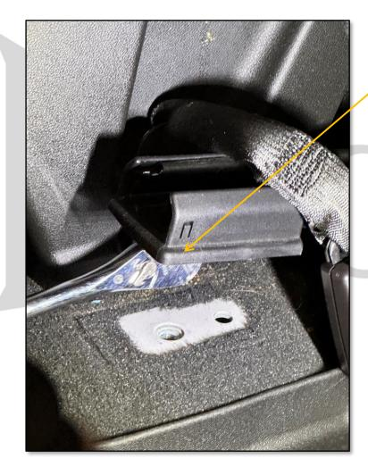
REMOVE FRONT AND REAR MOUNTING BOLTS FOR CENTER SEAT. SEAT THEN WILL HAVE TO BE LIFTED SLIGHTLY TO CLEAR ALIGNMENT PINS. MOVE SEAT TO THE BACK TO MAKE ROOM FOR CONSOLE.
