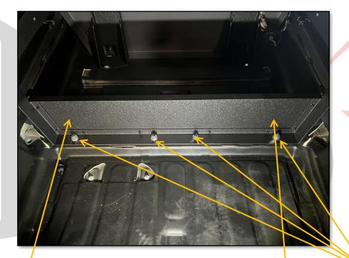
\*\*\* NOTE: MOUNT SHOWN INSTALLED REVERSED FOR CLARITY – THIS MOUNT WILL BE INSTALLED WITH FILLER PANEL IN FRONT (TOWARDS REAR HATCH). \*\*\*
