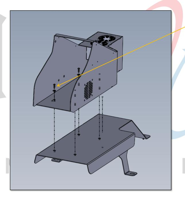
ATTACH CONSOLE TO FLOOR PLATE USING PROVIDED SCREWS AND WASHERS. BOLT TO PRE-INSTALLED NUTSERTS AND ADJUST POSITION TO CLOSE GAP WITH DASH PANELS.
