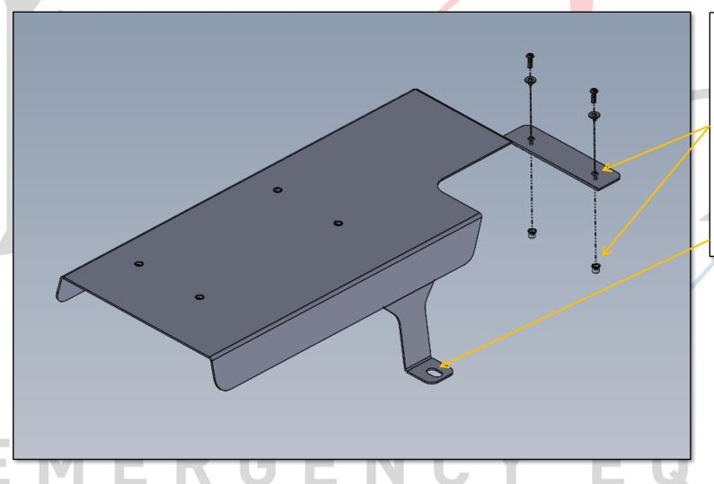
PLACE FLOOR PLATE OVER FACTORY MOUNTING HOLES
