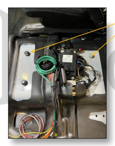
LOOSEN FACTORY BOLTS ENOUGH TO SLIDE MOUNTING FEET UNDER, MAKE SURE ARROWS ON MOUNTING FEET POINT TOWARDS FRONT OF VEHICLE.
