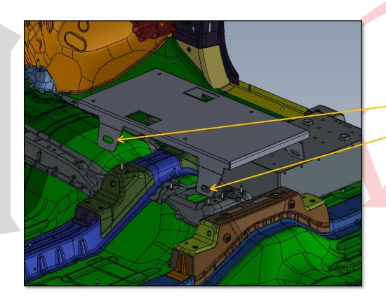
PLACE FLOOR PLATE OVER HOLES USED FOR FACTORY CONSOLE.
