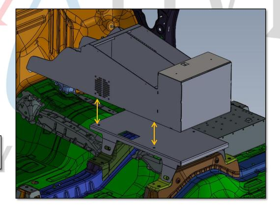
SECURE CONSOLE TO FLOORPLATE WITH PROVIDED HARDWARE
