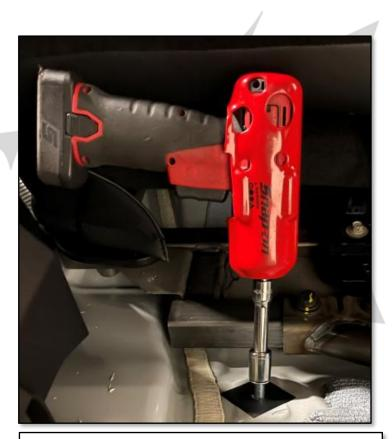
USING AN IMPACT TOOL AND THE SELF-TAPPING BOLT (SUPPLIED), THREAD THE FACTORY HOLE.
