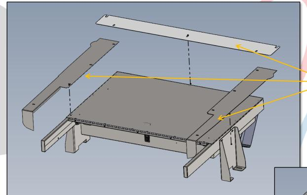
LAY FLAT FRONT COVER OVER FRAME, THEN LAY REAR FILLER PLATE AND SIDE WINGS. FASTEN USING SUPPLIED HARDWARE, AND INSTALL FINAL SOCKET HEAD CAP SCREWS TO WING SUPPORTS.
