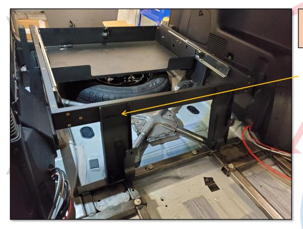
INSERT (2) 10-32 BUTTON HEAD CAP SCREWS TO SIDE MOUNTS INTO FRAME AND TIGHTEN, THEN INSTALL DRAWER USING SUPPLIED HARDWARE PLEASE NOTE THE FOLLOWING CAN BE DONE WITH THE DRAWER AND FRAME ASSEMBLED, OR YOU CAN REMOVE THE SLIDES AND DRAWER FROM THE FRAME, AND RE-INSTALL THE DRAWER WHEN DONE.
