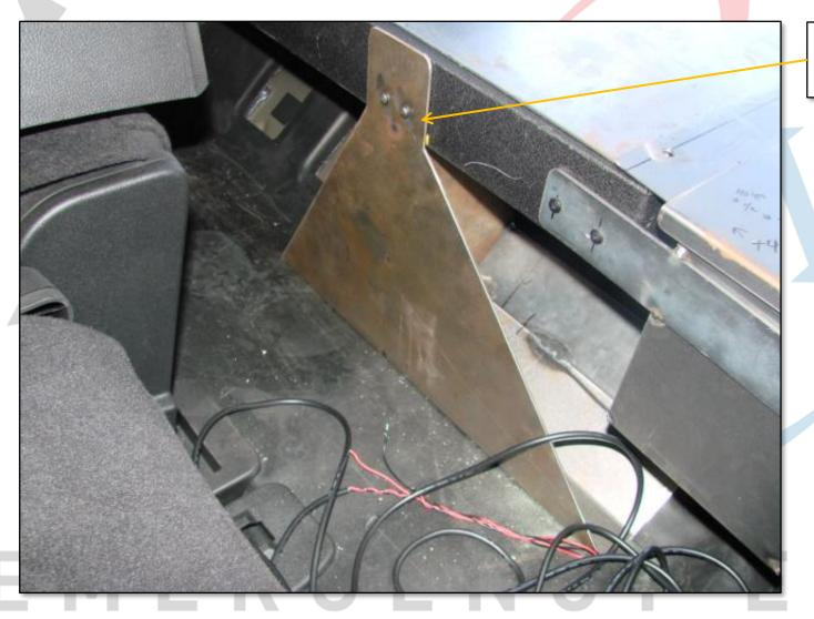
ATTACH FRAME TO FEET WITH PROVIDED SCREWS
