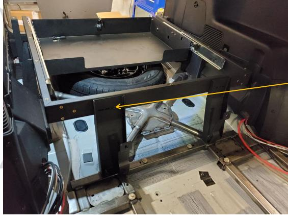
INSERT (2) 10-32 BUTTON HEAD CAP SCREWS TO SIDE MOUNTS INTO FRAME AND TIGHTEN, THEN INSTALL DRAWER USING SUPPLIED HARDWARE PLEASE NOTE THE FOLLOWING CAN BE DONE WITH THE DRAWER AND FRAME ASSEMBLED, OR YOU CAN REMOVE THE SLIDES AND DRAWER FROM THE FRAME, THEN RE-INSTALL THE DRAWER WHEN DONE.
