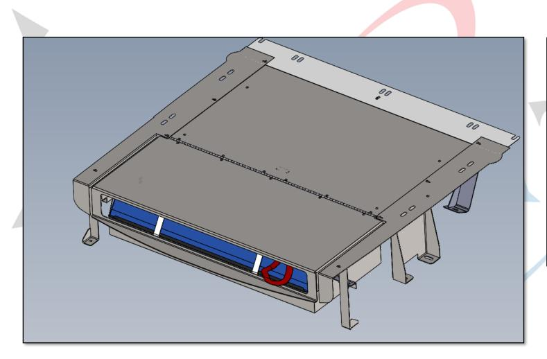
INSTALLATION OF STOP STICK FALSE FLOOR IN FORD PIU20
