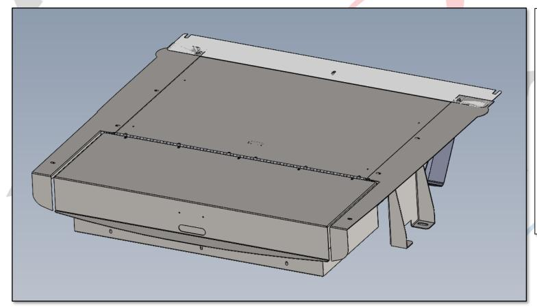
INSTALLATION OF FALSE FLOOR IN FORD PIU20
