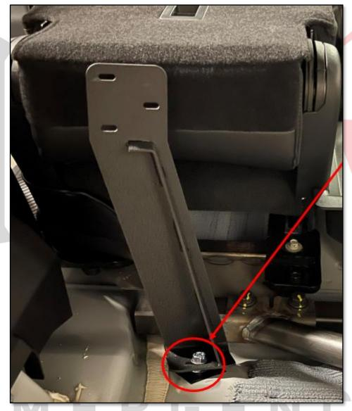
REMOVE INSTALLED BOLT, INSTALL AND SECURE BRACKET WITH SAME BOLT.
