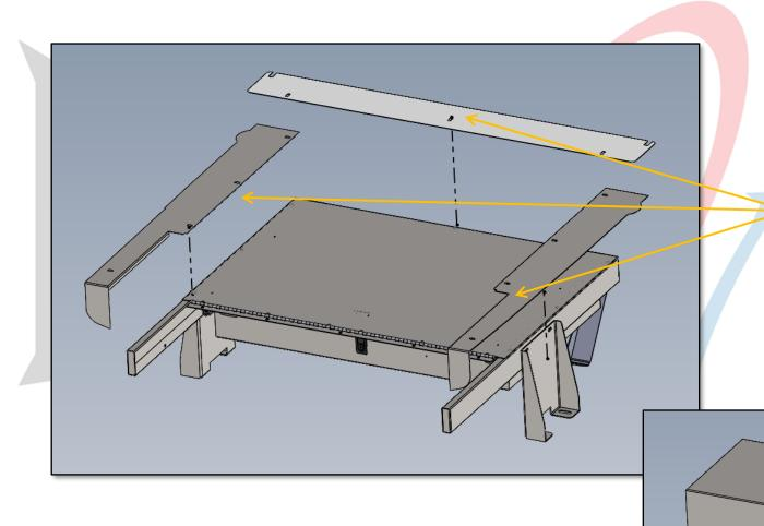
LAY FLAT FRONT COVER OVER FRAME, THEN LAY REAR FILLER PLATE AND SIDE WINGS. FASTEN USING SUPPLIED HARDWARE, AND INSTALL FINAL SOCKET HEAD CAP SCREWS TO WING SUPPORTS.
