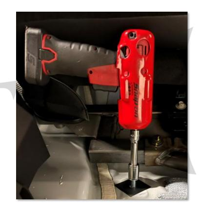
USING AN IMPACT TOOL AND THE SELF-TAPPING BOLT (SUPPLIED), THREAD THE FACTORY HOLE.
