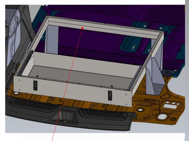
PLACE FRAME AND DRAWER ASSEMBLY INTO VEHICLE.
