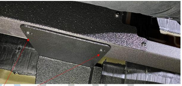
**INSTALL SUPPLIED 10-32** BHCS INTO ALL MOUNTING **BRACKETS ON FRAME**
