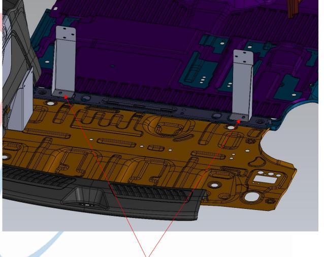
USE A UTILITY KNIFE TO CUT ALONG THE FLOOR MAT ON THE 3<sup>RD</sup> ROW SEAT RAIL. REMOVE TRIMMED PIECE. USING HARDWARE PROVIDED, INSTALL TWO FRONT MOUNTING FEET TO VEHICLE.
