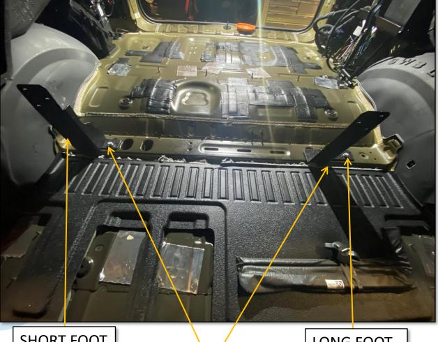
USE A UTILITY KNIFE TO CUT ALONG THE FLOOR MAT ON THE 3<sup>RD</sup> ROW SEAT RAIL. REMOVE TRIMMED PIECE. **SHORT FOOT**
