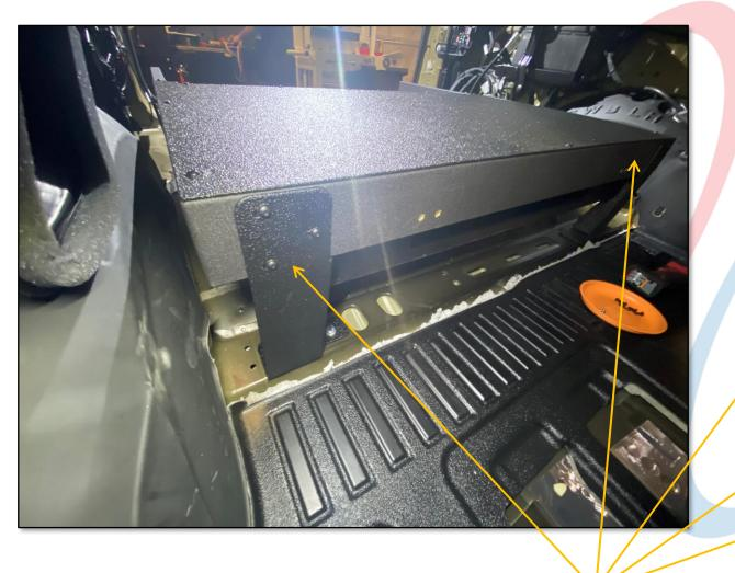
INSTALL SUPPLIED 10-32 BHCS INTO ALL MOUNTING BRACKETS ON FRAME
