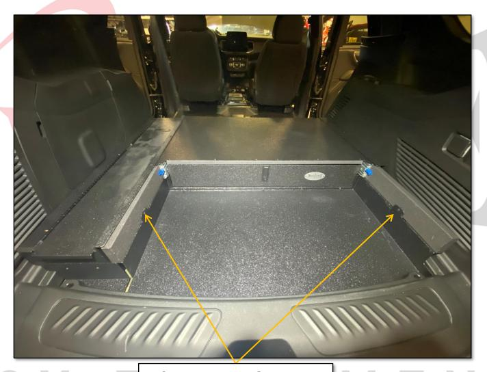
INSTALL THE TWO FLAT HEAD SCREWS INTO THESE EARS INTO THE FRAME
