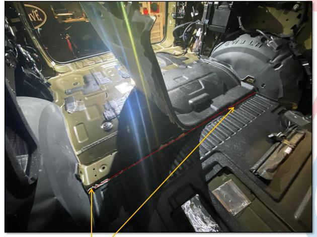
USE A UTILITY KNIFE TO CUT ALONG THE FLOOR MAT ON THE 3<sup>RD</sup> ROW SEAT RAIL. REMOVE TRIMMED PIECE.
