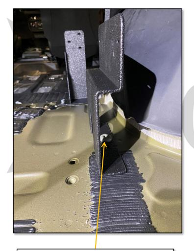
INSTALL PASSENGER REAR FOOT USING REMOVED FACTORY BOLT
