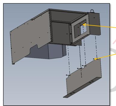
STEP 4) INSTALL TRIM PANEL TO INSIDE OF FRAME USING PROVIDED SELF-TAPPING SCREWS
