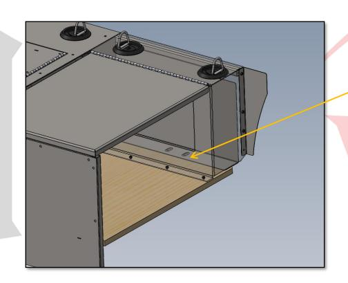
STEP 6) SECURE ASSEMBLY TO REAR FLOOR HOLES WITH FACTORY HARDWARE (PANEL GHOSTED FOR CLARITY)
