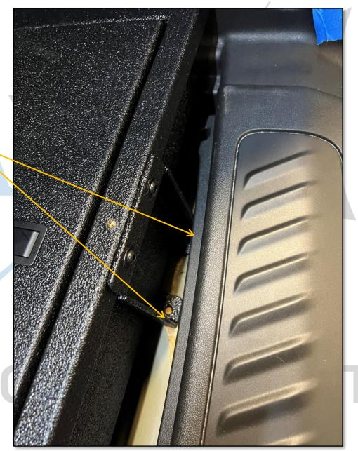
SLIDE FLOOR TOWARD FRONT ON MOUNTS, REMOVE THE RUBBER FROM THE VEHICLE FLOOR, AND DRILL AND INSTALL NUTSERTS INTO VEHICLE FLOOR. REMOVAL OF REAR LOWER TRIM WILL MAKE THIS EASIER.
