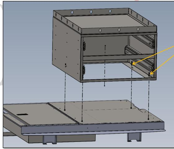
MOUNT DUAL DRAWER UNIT TO PRE-INSTALLED NUTSERTS USING SUPPLIED 1/4-20 HARDWARE
