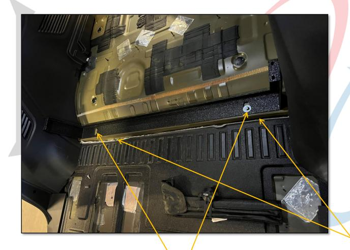
USING PROVIDED 3/8" BOLTS AND WASHERS, INSTALL REAR STRAP INTO CAR, BEND IN STRAP WILL BE TOWARDS REAR OF CAR. DO NOT TIGHTEN AT THIS POINT.
