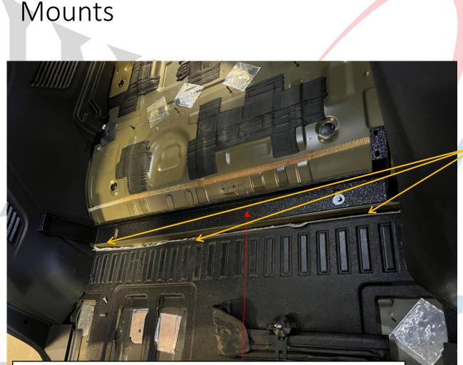
REMOVE FACTORY RUBBER FLOOR IN REAR OF VEHICLE.
