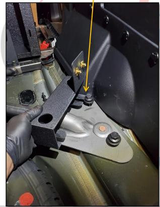
TIGHTEN BOLTS TO SECURE SIDE FEET, REPEAT FOR OPPOSITE SIDE
