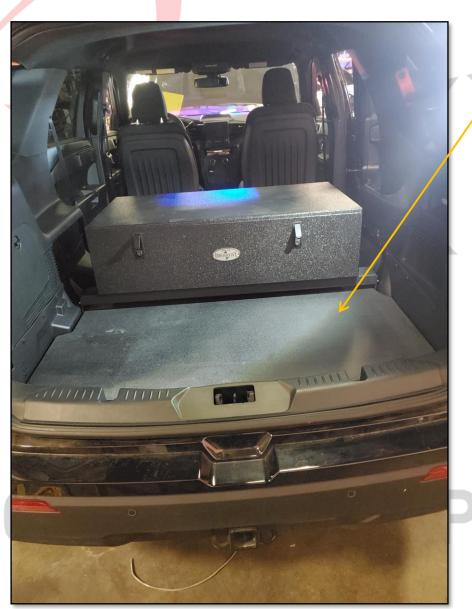
REINSTALL DRAWER IN BOX AND REPLACE SPARE TIRE COVER PANEL TO COMPLETE INSTALL
