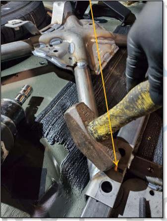
USING FACTORY HARDWARE, ATTACH FRONT FEET TO SUBFRAME AS SHOWN
