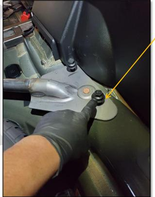
LOOSEN FACTORY BOLTS ON SIDE OF SUBFRAME, AND SLIDE SIDE MOUNTING FOOT INTO PLACE AS SHOWN
