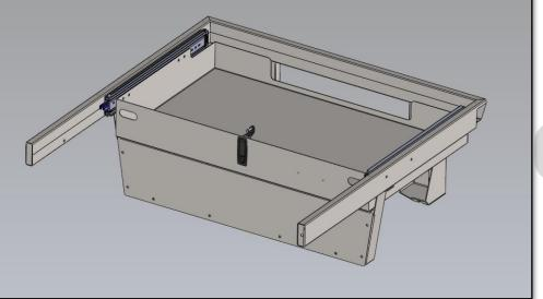
UTILIZING 10-32 SCREWS, INSTALL FRONT MOUNTING FEET AND REAR U BRACKET ONTO FRAME.
